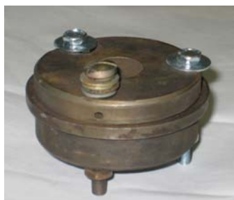
Figure 1. The container with rubber samples inside.
