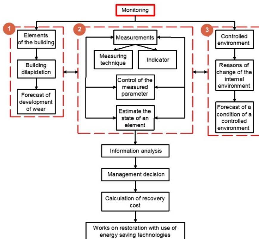
The block 2 carries out continuous tracking of temperature environment parameters in rooms and point out the comparison with their standard indicators developing multiple optimizing models of technical condition of buildings, thereby increasing economic and social efficiency of the overhauls.
