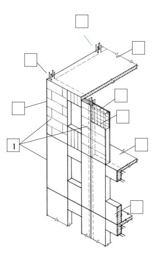
**Figure 1**. Section of a biding wall erected in compliance with' the proposed method, general view
