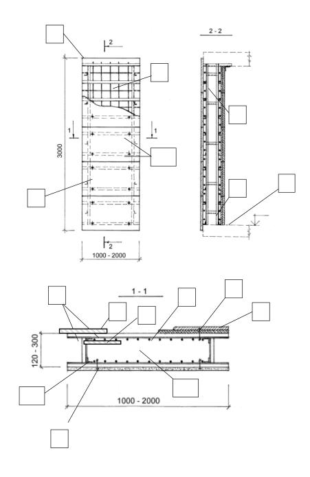
Figure 2. Light hollow wall element, sectional view
